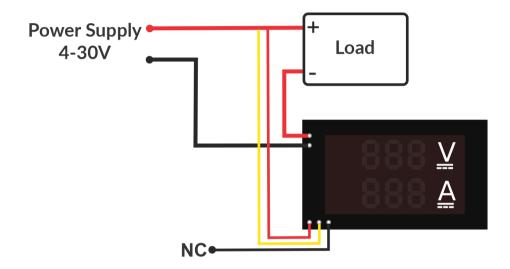
This is the typical application where module is connected on the same power supply as the load. The maximum voltage should not exceed 30V.
