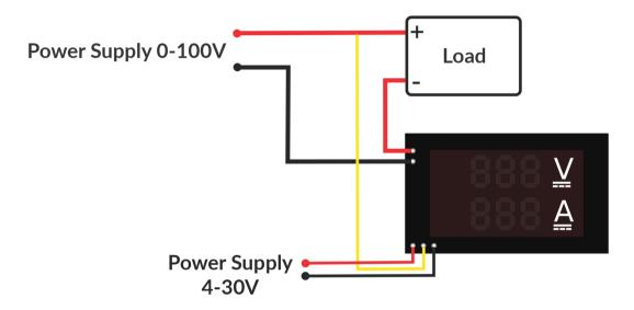
This type of wiring is used when power supply voltage is more than 30V and up to 100V. In that case, external power supply for the module is required.
