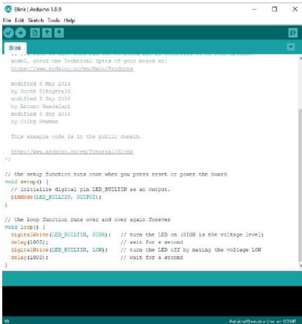
The image shows a screenshot of the Arduino IDE interface. The window title is "Blink | Arduino 1.8.9". The menu bar includes "File", "Edit", "Sketch", "Tools", and "Help". Below the menu bar is a toolbar with icons for check, run, upload, and download. The main text area contains the following code:
