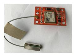
GY-NEO6MV2 board features the u-blox NEO-6M GPS module with antenna and built-in EEPROM. This is compatible with various flight controller boards designed to work with a GPS module.
