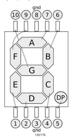
0-9 ten digits correspond with each segment are as follows (the following table applies common cathode seven segment display device, if you are using a common anode, the table should be replaced every 1 0 0 should all replaced by 1):
