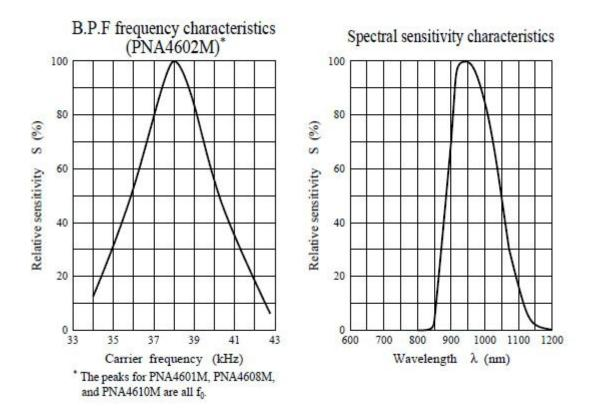
As you can see from these datasheet graphs, the peak frequency detection is at 38 KHz and the peak LED color is 940 nm. You can use from about 35 KHz to 41 KHz but the sensitivity will drop off so that it won't detect as well from afar. Likewise, you can use 850 to 1100 nm LEDs but they won't work as well as 900 to 1000nm so make sure to get matching LEDs! Check the datasheet for your IR LED to verify the wavelength.
