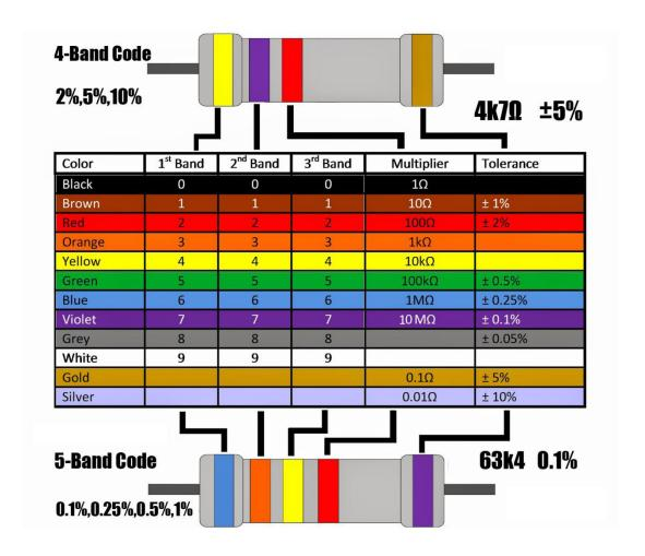
Unlike LEDs, resistors do not have a positive and negative lead. They can be connected either way around.
