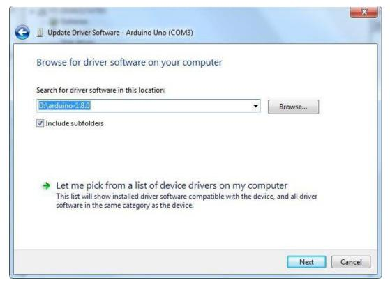
Click 'Next' and you may get a security warning, if so, allow the software to be installed. Once the software has been installed, you will get a confirmation message.
