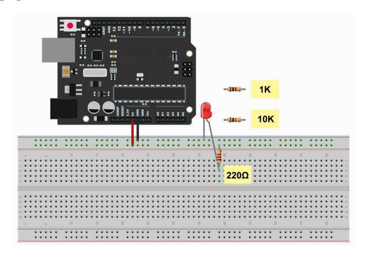
The UNO is a convenient source of 5 volts, which we will use to provide power to the LED and the resistor. You do not need to do anything with your UNO, except to plug it into a USB cable.
