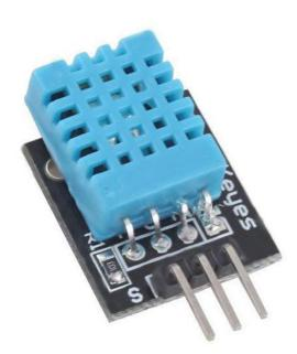
DHT11 digital temperature and humidity sensor is a composite Sensor which contains a calibrated digital signal output of the temperature and humidity. The dedicated digital modules collection technology and the temperature and humidity sensing technology are applied to ensure that the product has high reliability and
