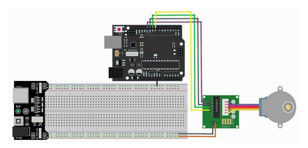
We are using 4 pins to control the Stepper.
