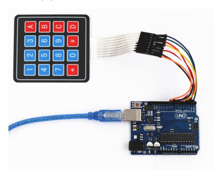
With this code, once we press a key on the keypad, it should show up on the serial monitor of the Arduino software once the code is compiled and uploaded to the UNO R3 board.
