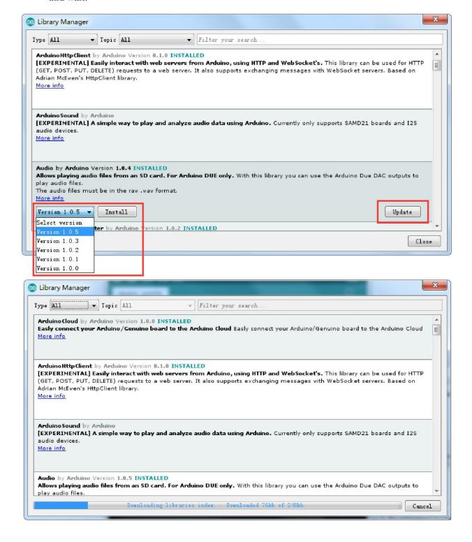
Finally click on install and wait for the IDE to install the new library. Downloading may take time depending on your connection speed. Once it has finished, an Installed tag should appear next to the Bridge library. You can close the library manager.
