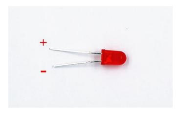
If you do not use a resistor with an LED, then it may well be destroyed almost immediately, as too much current will flow through, heating it and destroying the 'junction' where the light is produced.
