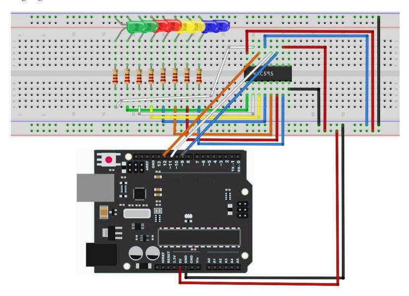
As we have eight LEDs and eight resistors to connect, there are actually quite a few connections to be made.
